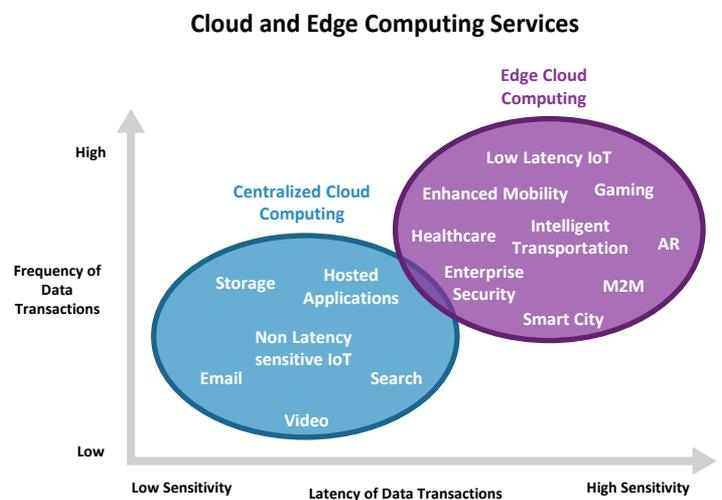
Figure 3 illustrates the key differences (data frequency and latency) between cloud and edge computing applications. Source: ECI – The Elastic Network “Enriching Edge Services With Virtualized Transport”, Hayam Porat, CTO
